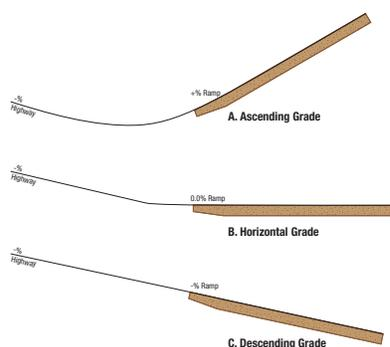
Vehicle escape ramps are designed and constructed in areas where steep grades exist to provide a location for out-of-control vehicles to come to a safe stop. They save the lives of the vehicle operators as well as reduce property damage.
